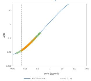
Representation of sample reading with IL-17A Advantage PLUS assay, the dots show 100 individual plasma (orange) and serum samples (green).
